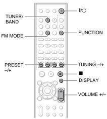
1 Press FUNCTION repeatedly until FM or AM appears in the front panel display.
